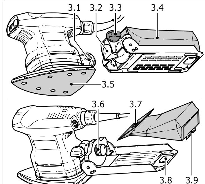
The machines are fitted with inbuilt extraction as standard. The sanding dust is extracted through suction openings in the sanding base (3.5) and trapped in the turbo-filter (3.4).
